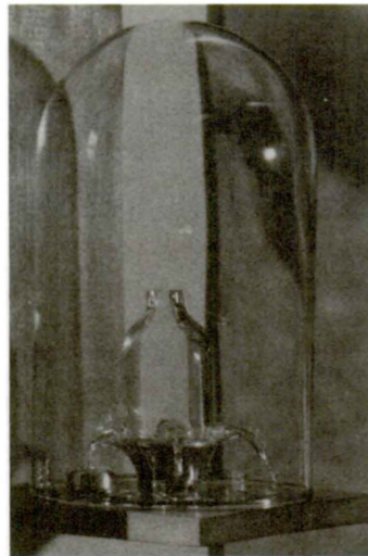
Fig. 2. Cavalli mercury seismoscope (1784). Historical copy made by SGA from description and drawings (Cavalli, 1785). A clockwork version of the instrument was also designed by Cavalli (Ferrari, 1992b, 42-46).
